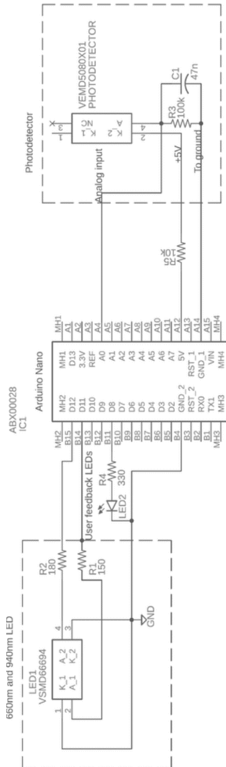
Figure 5.5: Circuit design of the pulse oximeter device.
