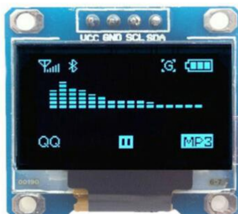
Figure 5.8: I2C battery operated and Arduino compatible LCD screen (Ebay, 2020).
