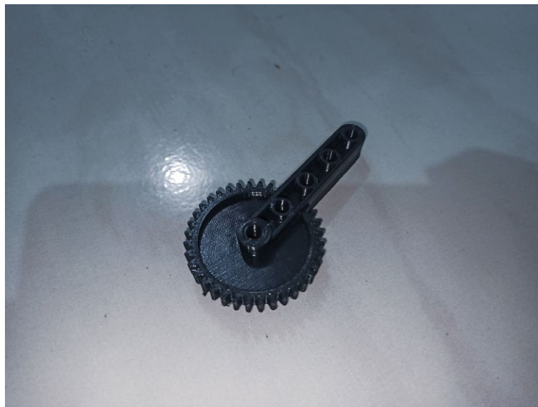
Figure 5-2. 3D printed claw gear linkage.
