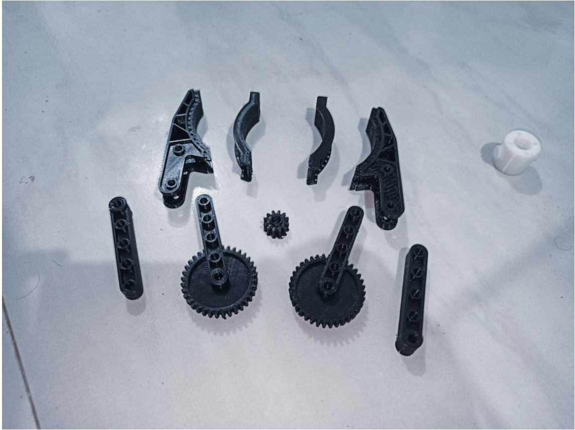
Figure 5-11. The 3D printed parts required to be assembled to fabricate the gripper arm.
