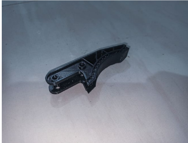
Figure 5-9. 3D printed claw gripper.
