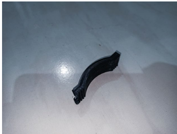
Figure 5-10. 3D printed claw finger.
