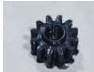
Figure 5-4. 3D printed gear connected to the stepper.
