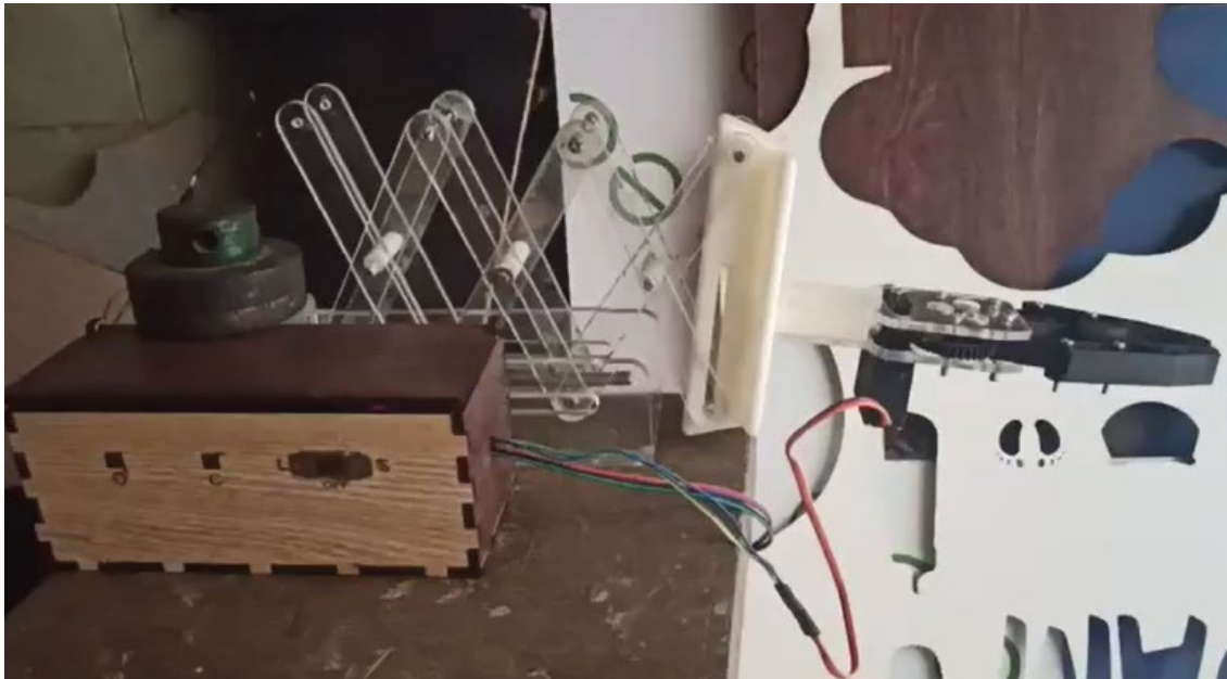
Figure 5-12. Gripper Arm had been 3D printed and assembled (in the retraction mode).
