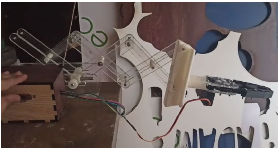
Figure 5-13. Gripper Arm had been 3D printed and assembled (in the extension mode).
