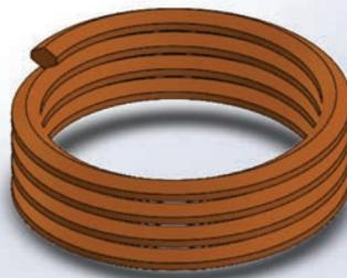
Figure 3-6. 3D model for the spring of the flow control valve.
