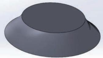
Figure 3-8. 3D model for the diaphragm of the flow control valve.
