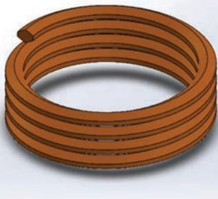
Figure 3-6. 3D model for the spring of the flow control valve.
